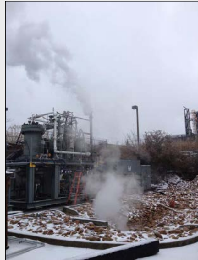
Georgia Tech University 100kWth Plant Operating pressure: 30 Bar Main use: Coal testing Not in operation
